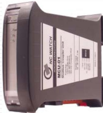
The MCU has an RS-485 port (dual connectors A and B, for cascading purposes), fiber connectors and an RS-232 port. Used ports are selected with jumpers in an MCU. Bias voltages and bus terminators have their own DIP switches. In the front panel there is a power LED and status indication LEDs for communication. The MCU is DIN rail mountable.
